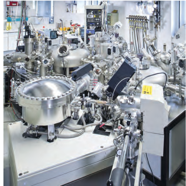
Fig. 5: The ultrahigh vacuum cluster - a modern technique for analysing the surface of materials - is one of the topics presented at the Max Planck Science Gallery.
