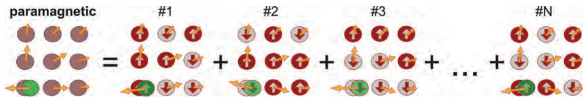
Fig. 1: Sketch of the SSA procedure. The effective forces at finite magnetic temperatures are obtained from a set of disordered magnetic configurations.
