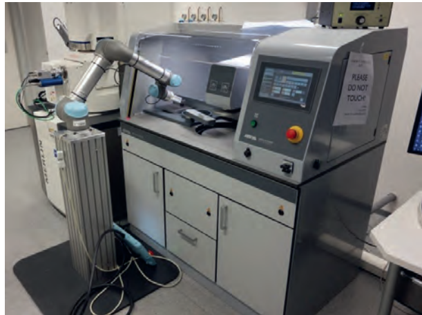
Fig. 1: Combination of the Saphir X-Change polishing automata (the main gray box), the UR5 cobot (in the front) and the Zeiss Merlin SEM (behind both in the background). The cobot is currently picking up a sample which has been placed on an exchange table by the polishing automata. It will subsequently open the microscope door, place the sample in the microscope and close the door again.
