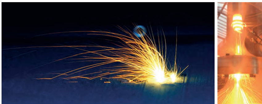
Fig. 1: Image of the SLM process during operation (left). The “sparks” captured are the typical ejected powder particles that are carried away from the melt pool by the inert gas cross jet. On the right hand side, the gas atomization process is shown (initial experiments).
